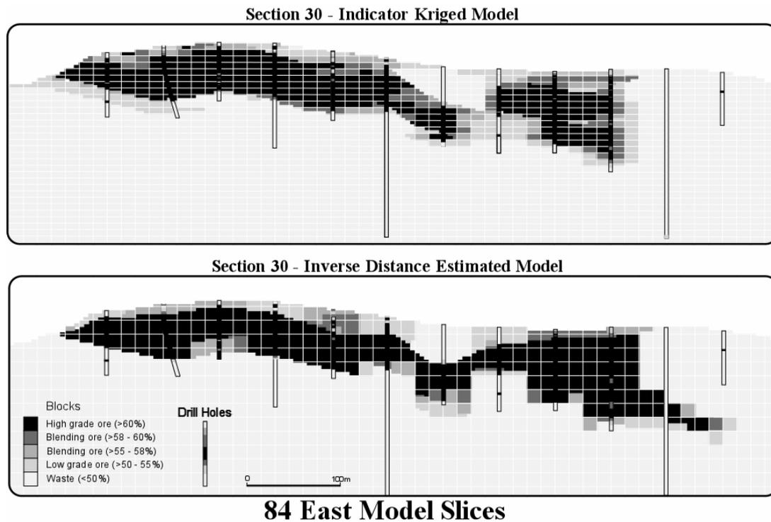
*Figure 7. 84 East deposit model slices: Section 30 of Median Indicator Kriged Model and Section 30 of Inverse Distance Estimated Model.*
